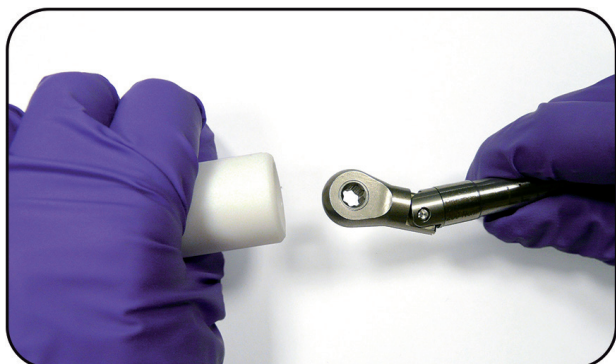
To reverse this disengagement and be able to use it again, insert it into the plastic reset tube.
