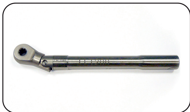
Wrench that has been disengaged upon reaching 200 Ncm.
